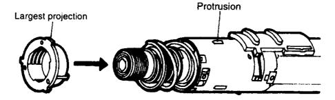
4. When assembling the clutch handle, position the clutch handle with position number"2" towards the largest protrusion of adjusting screw.
