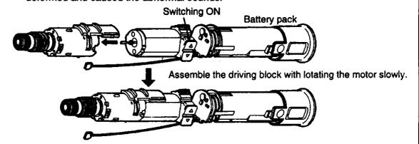
Insert the torque detection PCB into the groove of driving block.
