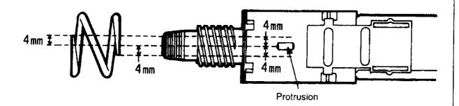
When assembling the adjusting screw, align the protrusion of the driving block with the largest protrusion of the adjusting screw.
